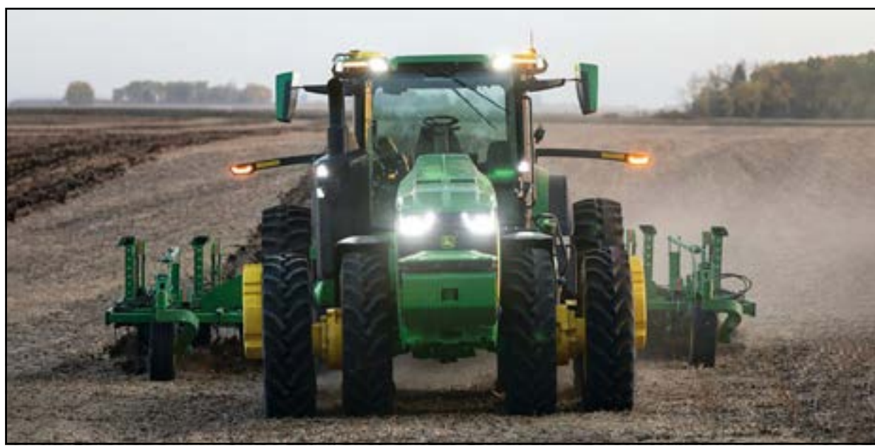
JOHN DEER WILL PLOW FOR YOU —Full auto vehicles already working—on farms. John Deere is producing a number of self-driving tractors. It is easier to keep them on the straight and narrow than self-driving cars because there is no other traffic or surprise obstacles in the field.
